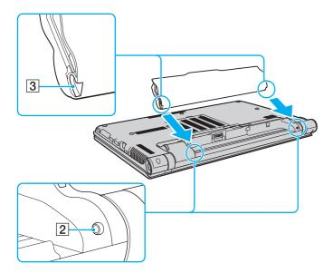
4 Push the battery pack down into the compartment until it clicks into place.
